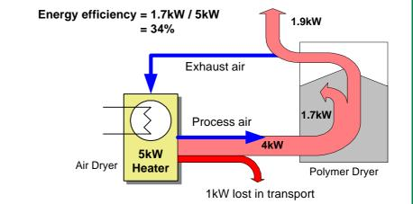
Energy flow in a conventional drying system - only 34% of the total input energy is used to heat and dry the polymer. The rest of the input energy is lost before or after drying.
