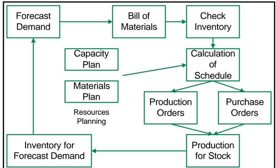
*The basic MRPII flow chart for production planning and control. The process is highly computerised and is sometimes too inflexible for the production of custom items such as windows. The system is excellent for items made up of many discrete parts (such as engines) but can fail if inventory accuracy is not adequate.*
