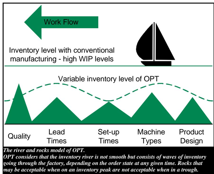
The location and management of bottlenecks is the heart of OPT. An hour saved at a bottleneck is an hour saved for the whole system but an hour saved on a non-bottleneck machine simply increases inventory and does nothing to improve throughput. It is wasted effort.
