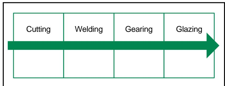
*Work flow in the conventional factory. Work moves around the factory in a long linear flow. There is little attempt to minimise the distance travelled (a good indicator of the time taken to produce the product), handling activity is high, WIP is high and balancing of the line is a continual struggle as the product mix changes from day to day.*
