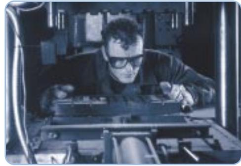
A company producing components for manufacturers of office equipment has used statistical techniques to confirm the existence of mould distortion. A subsequent change of press virtually eliminated scrap and achieved savings of more than £10 000/year.
