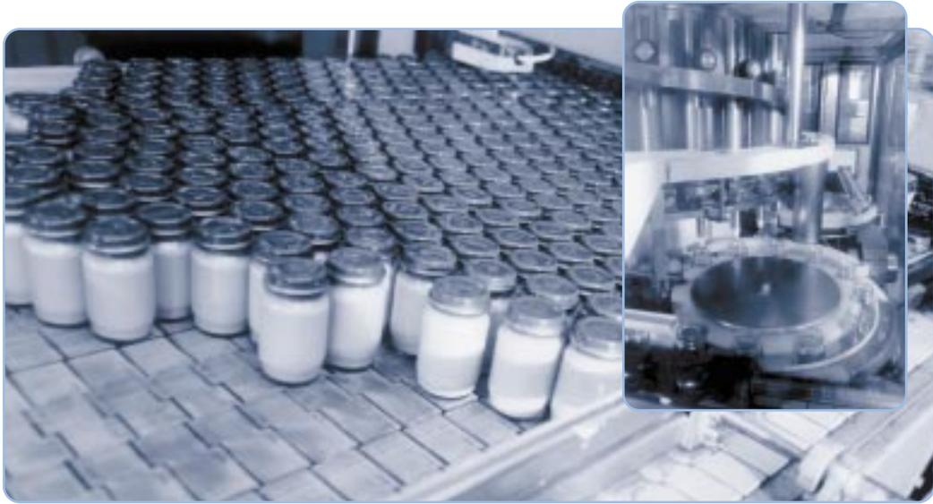
The company has made innovative use of its filling control records to reduce its levels of waste. It constructed a history of mean fill values and standard deviations, and used this to relate filling line **effects** to upstream process **causes**. As a result, improvements have been made in:
