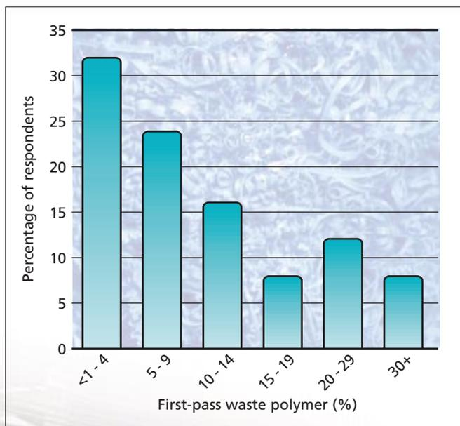
**Fig 5 Waste polymer generated in one pass by injection moulding operations**
