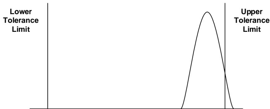
**The process spread is much less than the specified tolerances but out of tolerance parts are being produced. The machine needs adjustment.**
