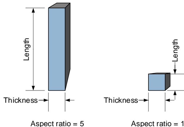
**Figure 3: The aspect ratio for two fillers, if the aspect ratio is greater than 200 the filler is more properly classed as a reinforcement.**
