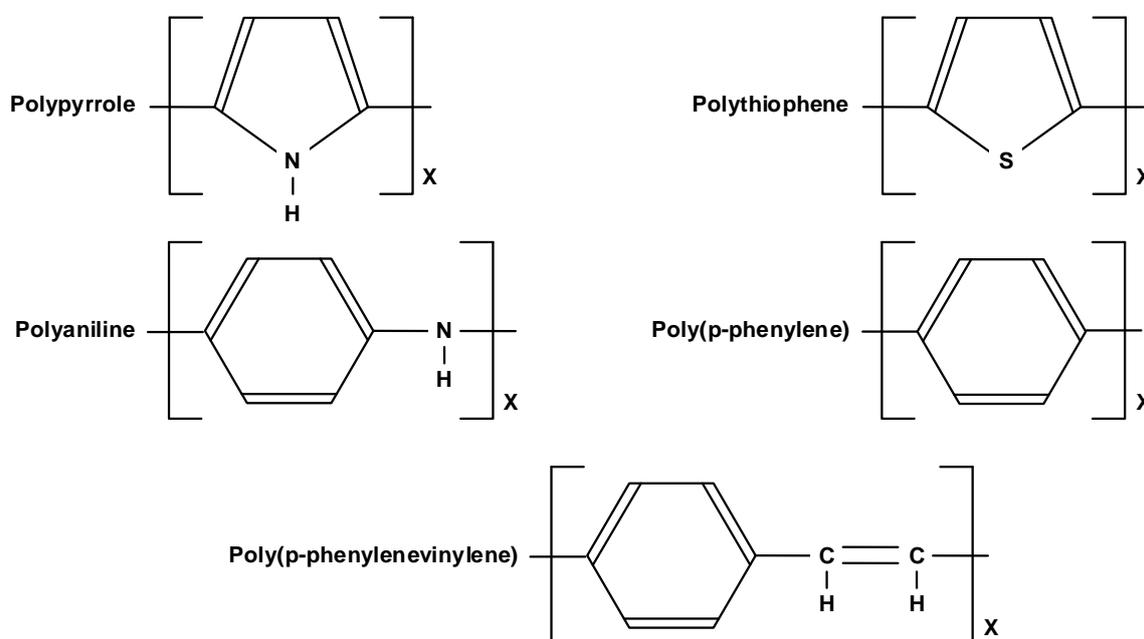
**Figure 6: Some of the polymers used in plastic electronics**
