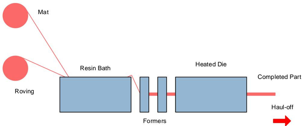
**Schematic of the pultrusion process**
