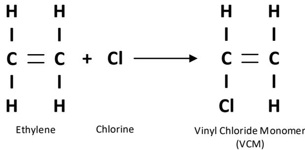
The VCM is then reacted by one of several methods so that it polymerises (or joins together) in long chains of about 1000 repeated units to form PVC.
